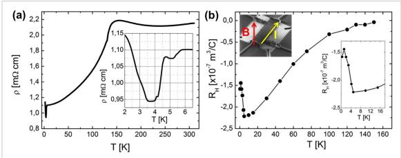
**Figure 1.** (a) Electrical resistivity from 2 to 320 K. Inset: enlarged view of the data between 2 and 8 K. (b)  $R_{\rm H}$  from 0.4 K to 150 K. Top-left inset: SEM images of the crystal with W electrical contacts. Right inset: zoom of the data between 0.4 K and 18 K.
