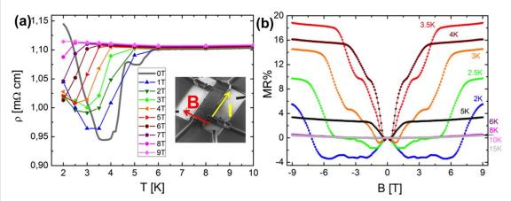
**Figure 2.** (a) Temperature dependence of the electrical resistivity between 2 and 10 K at selected magnetic fields B between 0 and 9 T applied perpendicular to the electrical current I, as shown in the inset. (b) B-dependence of the magnetoresistance from -9 T to 9 T at selected temperatures in the range 2–15 K.
